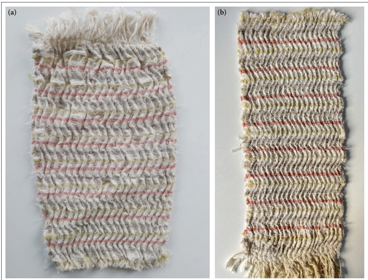
Figure 7. Design 1: (a) fabric woven on an automatic sample loom and (b) after the hot-water shrinkage process.
