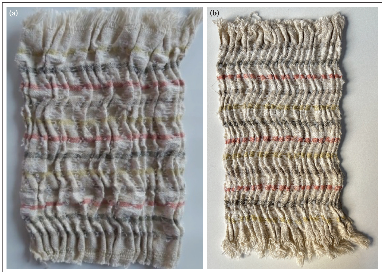
Figure 1. Design 1: (a) before the hot-water shrinkage process; (b) after the hot-water shrinkage process.
