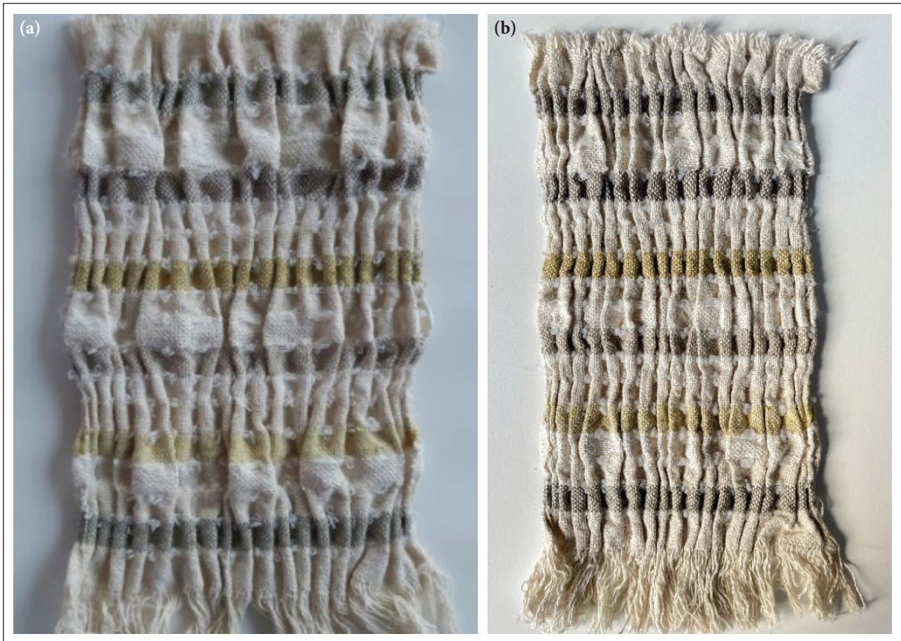
Figure 2. Design 2: (a) before the hot water shrinkage process, (b) after the hot water shrinkage process.
