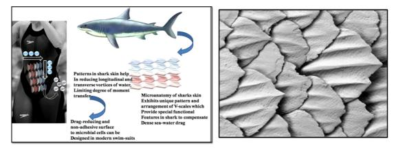
Image 8: Speedo's Swimsuit Design Based on the Structure of Sharkskin and its Detail Under the Microscope
